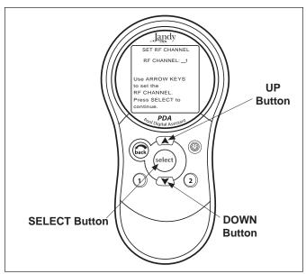
Figure 21. PDA Handheld Remote Channel Setup and Buttons
